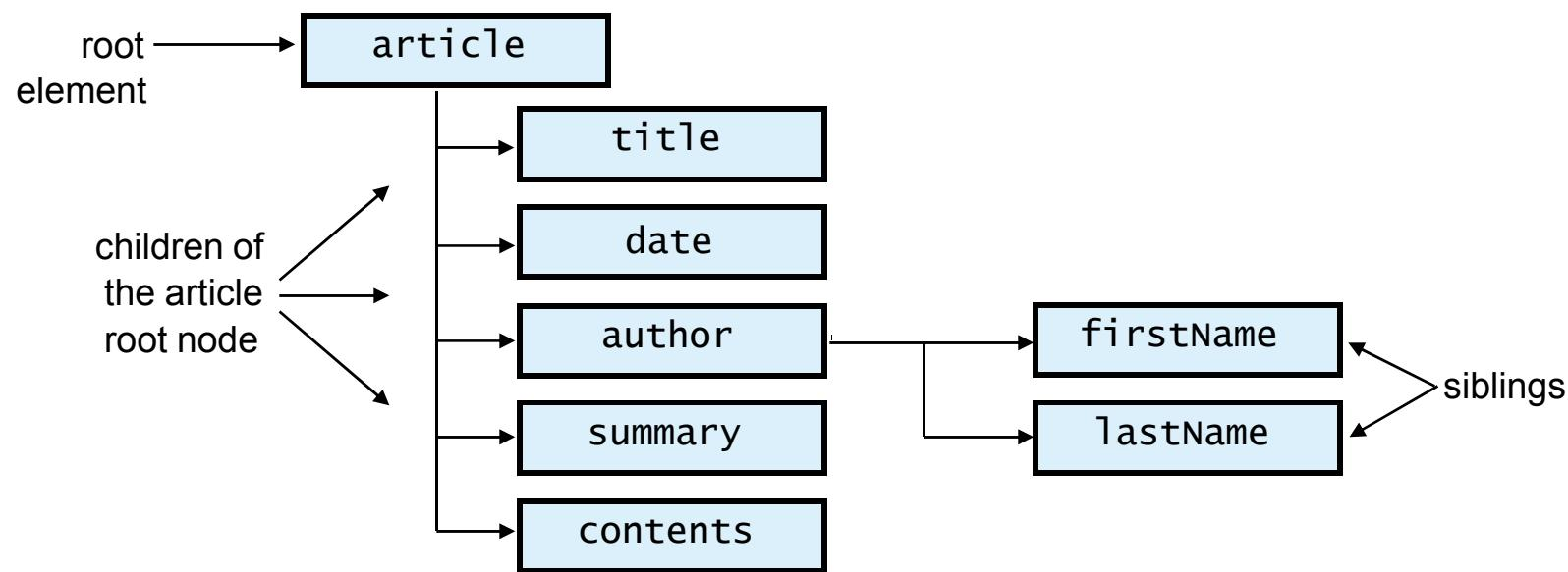
Fig. 20.18 Tree structure for `article.xml`.
